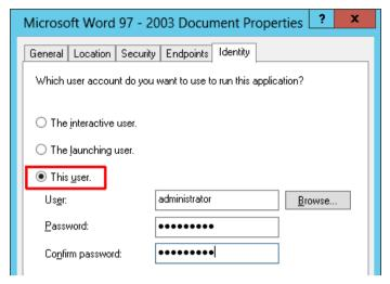
If only a single document type failed to convert in the Office Test and Diagnostics in step 1 above, such as Word documents (doc and docx), then you can change only DCOM permissions for that relevant application that failed.
