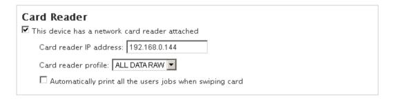
Checking Automatically print all users jobs when swiping card is a useful setting to enable if using card readers on simple network printers. Enabling this, and all the print jobs being held in EveryonePrint, will be released when user swipes their card.
